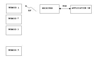
First level is the communication between the application sw and the receiver RF module.
