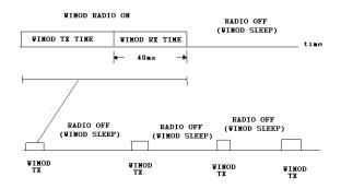
If a WIMOD does not receive at least one command from the master it goes in power down mode in order to save battery life. In power down mode WIMOD transmit a data packet every 8s.
